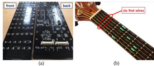
Figure 3. The fingerboard of the sensor-based guitar: (a) PCB embedded under the fingerboard, (b) the fingerboard with fret wires
