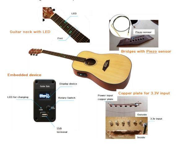
The main controller controls the lighting of the LED and performs the function of sensing the user of the performance information. Guitar bridges have a copper plate and a piezo sensor attached to them, and a voltage is applied to each guitar line through a copper plate to sense which frets the user puts on. A piezo sensor is also used to sense which guitar line the user has bounced.
